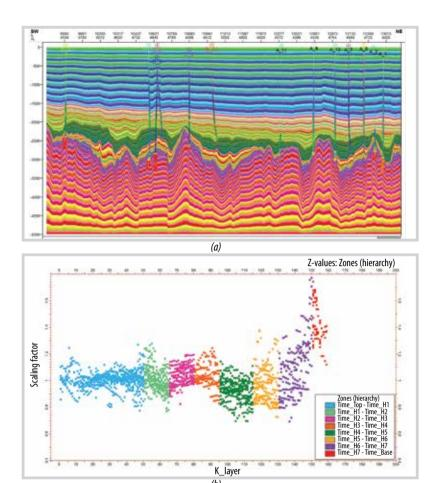
**Figure 3.** The scaling factor varies with the geological layer in the 3D structural model.
