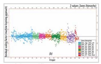
Figure 10. The residual scaling factor using scaling factor function (a) and residual scaling factor using machine learning approach (b).
