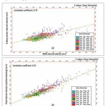
**Figure 9.** The correlation between scaling seismic interval velocity and well interval velocity (a), and the correlation between final interval velocity (machine learning approach) and well interval velocity (b).
