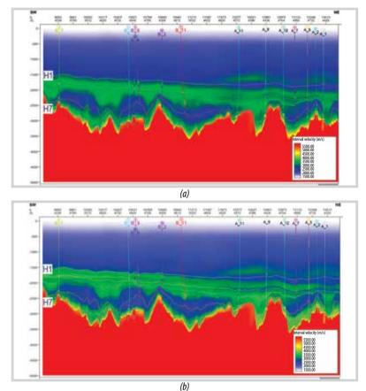
**Figure 8.** The scaling seismic interval velocity using scaling factor function (a) and the final interval velocity using machine learning approach (b).
